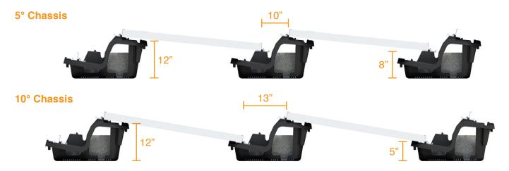
With 10-13" inter-row spacing, BX provides an 8-10% increase in power density compared with other ballasted systems—that's a capacity increase of 20% in a typical 50kW system. The BX Chassis geometry also offers more than 5" of clearance in the 10-degree configuration and 8" in the 5-degree configuration, enabling the system to avoid drain domes, roof saddles, and conduit supports.
