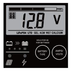
Press **BATTERY TYPE button** and hold for 3 seconds to go into your battery type selection mode, the battery type you select will be shown on the LCD meter, the default setting is AGM Battery; the controller will automatically memorize your battery type setting.
