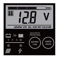
Caution: Prolonged connection with incorrect battery type setting may damage your battery.
