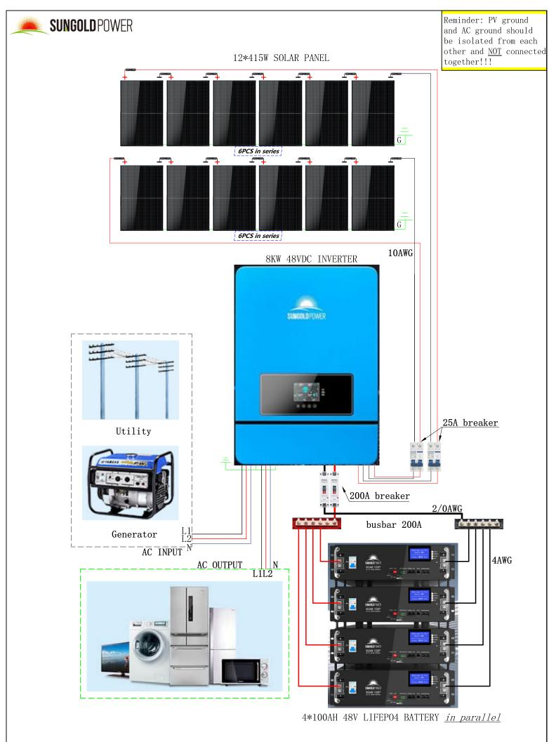
SOLAR KIT 12 X 415 WATTS SOLAR PANELS 4 X 5.12KWH LITHIUM BATTERY 8000W SOLAR INVERTER 48VDC 120V/240V
