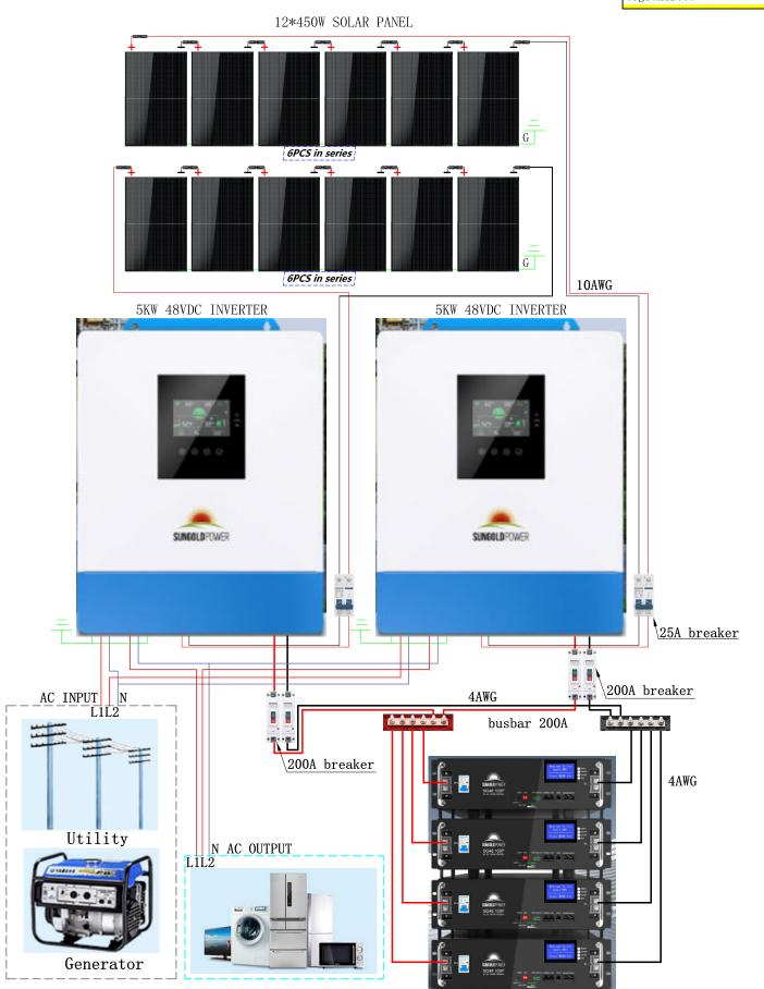
4\*100AH 48V LIFEPO4 BATTERY <u>in parallel</u>
