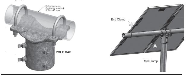
User supplies 4" schedule 40 steel pipe(s) for vertical pole and a 3" schedule 40 steel pipe for the horizontal beam. Calculation of the required horizontal beam length (L) in inches:  $L = 5 + (Q \times W) + ((Q-1) \times 1.28$  where Q = M module quantity, W = M width
